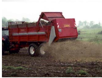
Fig.8.13: Poultry manure spreader with spreading table.
