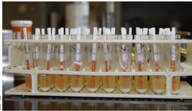
Fig.17.19: Many modern diagnostic assays are used as screening test to provide information of the presence or absence of specific pathogens, but normally they do not fully characterize the microorganism or presence of other pathogenic microorganisms. Some need little equipment investment, such as lateral flow.
