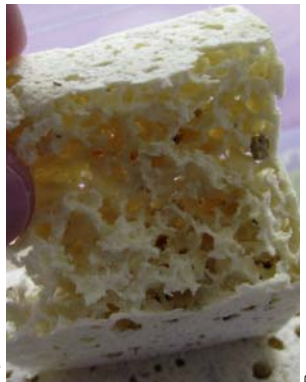
Fig.68.40, 68.41, 68.42 & 68.43: Alphitobius diaperinus (larvae). Darkling beetles are found in all kinds of structures, but more often in the walls. Larvae can drill holes in polystyrene foam, in fiberglass and insulation panels.
