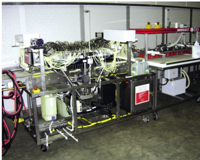
Fig.2.4: In ovo inoculation machine used at transfer from incubator to hatcher.
