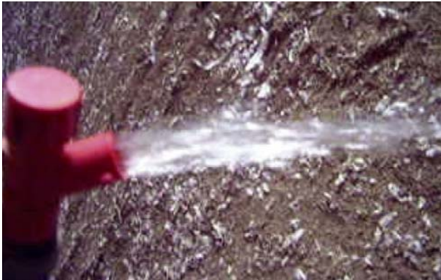
Fig.81.15 & 81.16: Not all products are effective in removing built up biofilm. On the left, this line was filled with a weak acid but as compared to the picture on the right (81.16), the solution did not remove any material. In 81.16, the water line was cleaned with a 3% solution of a 50% stabilized H 2 O 2 much more effective in disrupting and removing built up material in the system.
