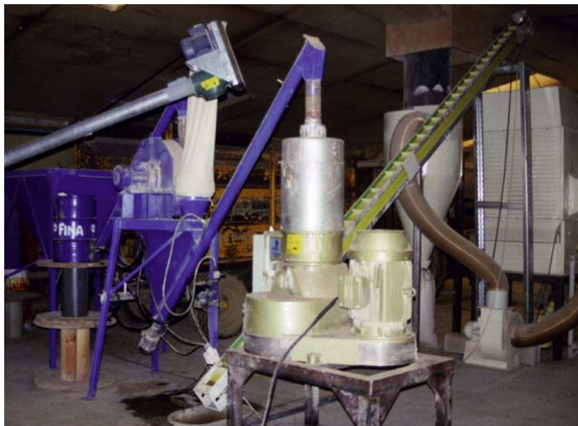
Fig.8.10: Granulation plant processing laying hen droppings.
