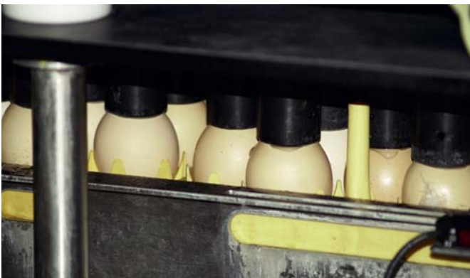
Fig.82.7: In ovo injections into embryonated eggs at transfer between setter and hatcher in the hatchery.
