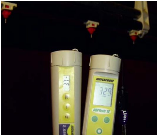
Fig.81.35: Measuring ORP is fast (less than 2 minutes) and provides information on free chlorine residual.
