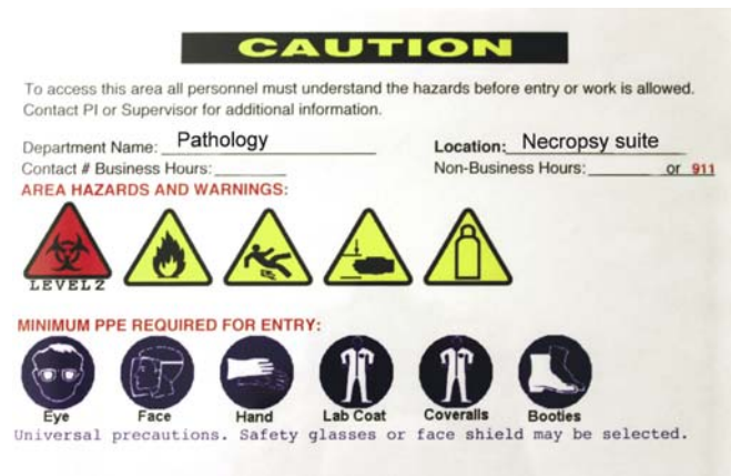
Fig.17.12: Laboratories should post warnings of hazardous areas as well as hazardous substances or conditions and recommended personal protective equipment.
